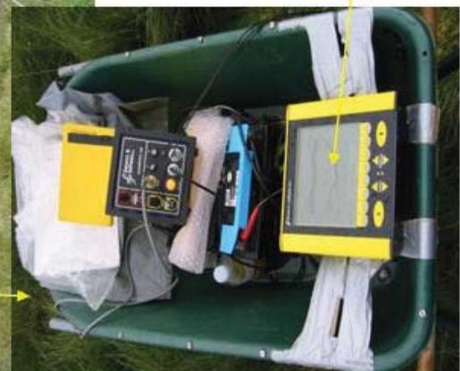
**GPR - 50 & 100 MHz antenna used to define thickness and lateral extent of peat deposits**
